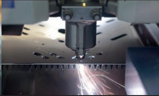
Computer controlled laser cutting the slots
