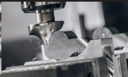
Milling of the positive fit in the lower part
