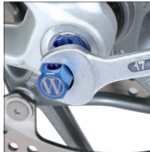
Usable as special tool for removing the front wheel and more.
