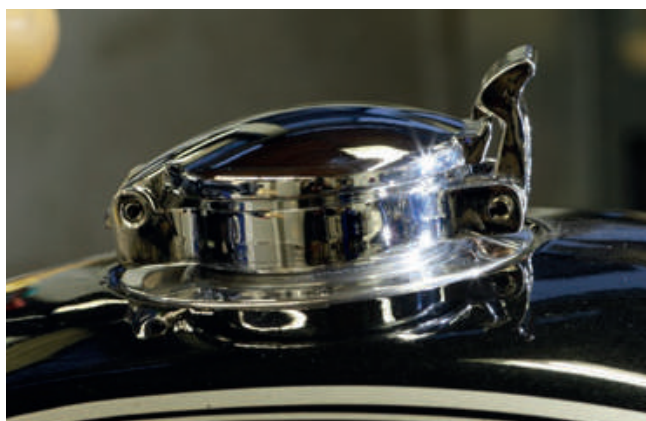
Aston tank cap with Adapter, here assembled on a R 100 R
