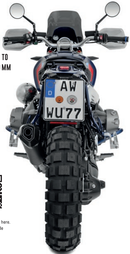
WITH CHASSIS RAISING KIT UP TO +70 MM
