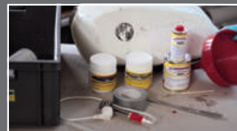
For tank refurbishment the repair set and an immersion heater is needed.
