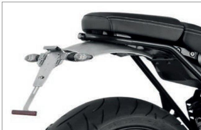
Tail conversion with integrated rear light »DEVILS-EYE« with license plate carrier »RETRO SPORT« in conjunction with original indicator set and aluminium mudguard
