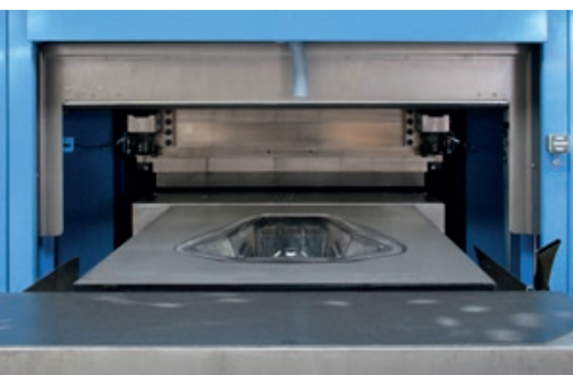
Hydroforming unit with die
