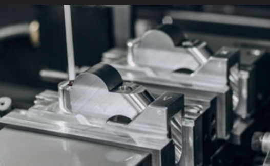
Computer-aided control with ruby stone tip
