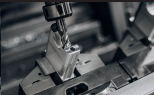
Drilling operation in the lower part of the handlebar riser
