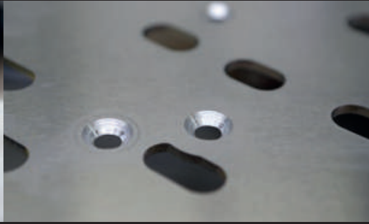
This allows flush bolting from below
