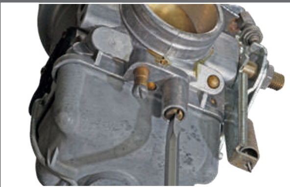
Turn Idle mixture screw (7) Carefully clockwise until fully closed
