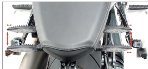
Indicator can be pulled in / out and mounted in two positions
