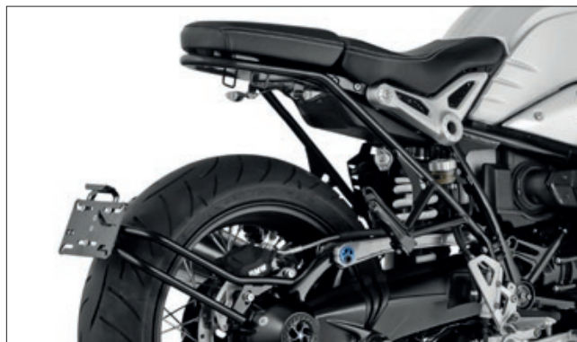
Tail conversion without rear light unit with license plate carrier »SWING« in conjunction with rear-/brake-/indicator combination Kellermann »MICRO RHOMBUS«
