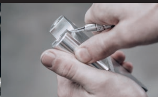
The edges are finished by the tool maker
