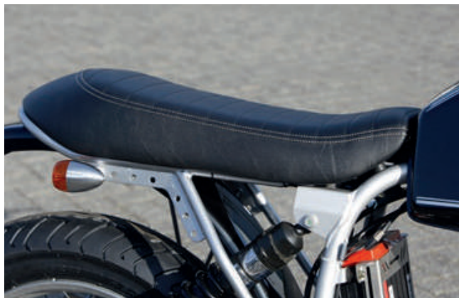
Seat »Pure« – features a circumferential light double seam
