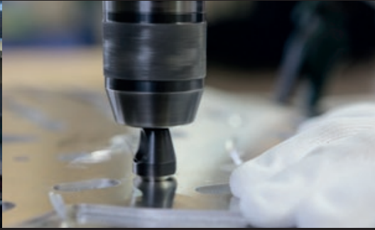
Mounting holes are finished with a countersink tool
