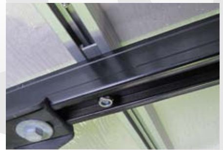
This diagram shows the rooftop tent bolted to a roof bar by drilling through the roof bar and attaching with bolts provided.
