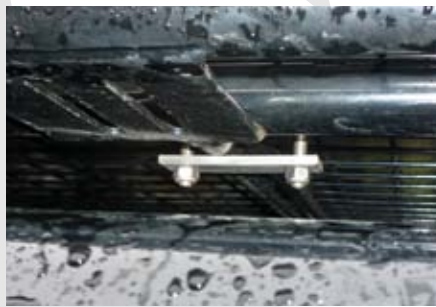
This diagram shows the rooftop tent clamped to a roof rack using clamp plate and bolts provided.
